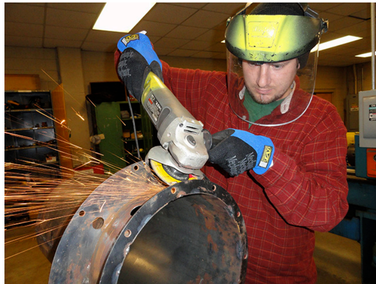
Sam Sink, graduate student, grinding on a gasifier reactor vessel
