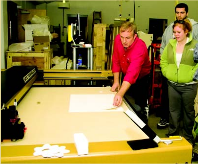
Jim Gossett of Gerber, demonstrates to students the use of the Gerber 3D Cutting table for cutting objects such as storage containers from drawings produced using CAD files.
